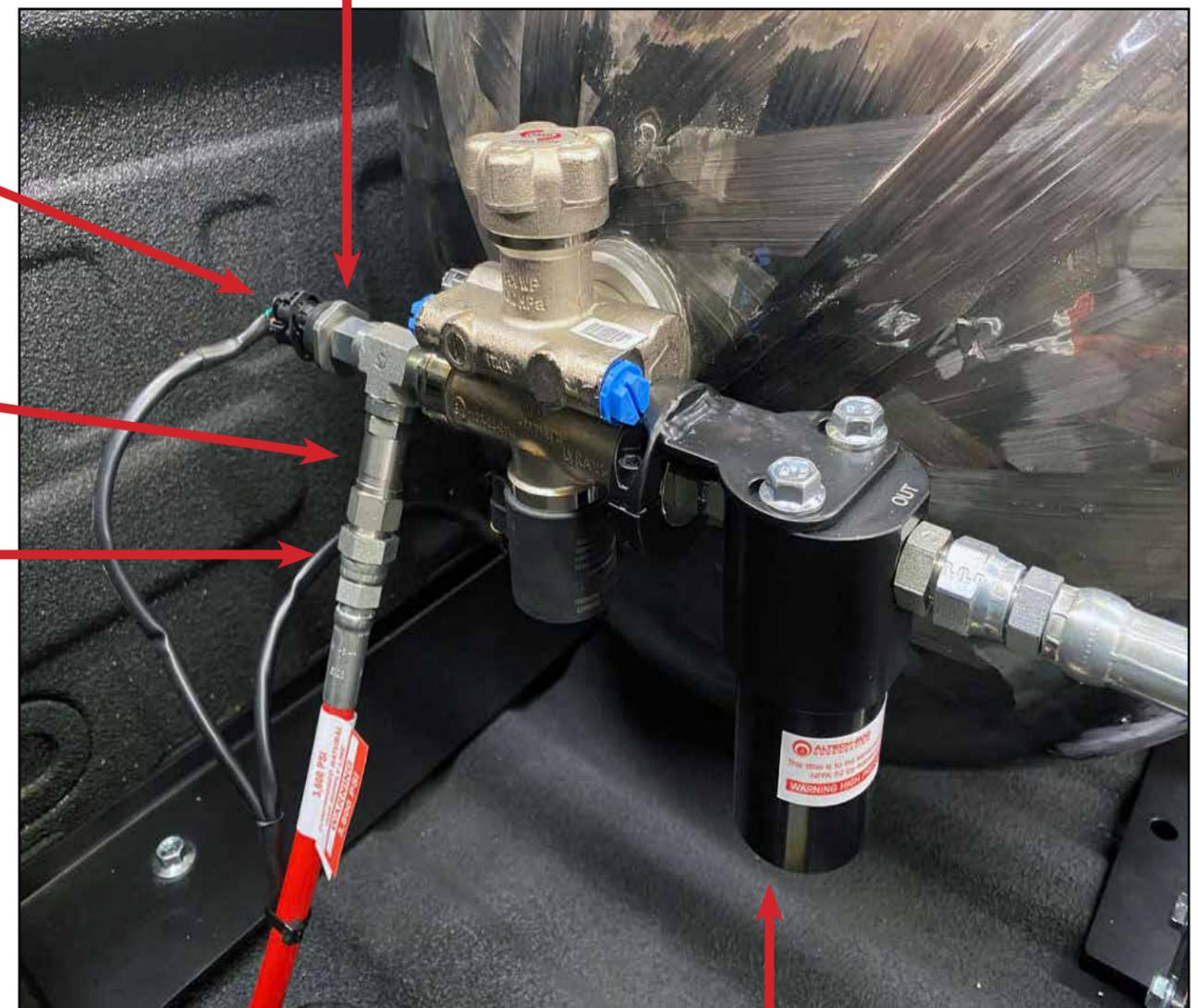
CNG Coalescing Fuel Filter Housing.
