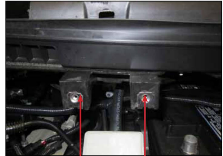
Remove these two tabs. Make a clean cut and flush with the plastic panel. Note: Picture displayed is for driver side, this must ONLY be done for the passenger side. **Do not touch the driver side tabs.**
